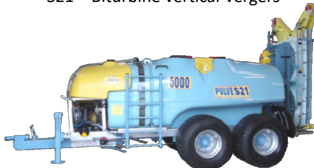
S21 – Biturbine vertical Vergers
